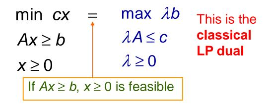
Note that the dual of the dual is the **primal** (i.e., the original LP).
