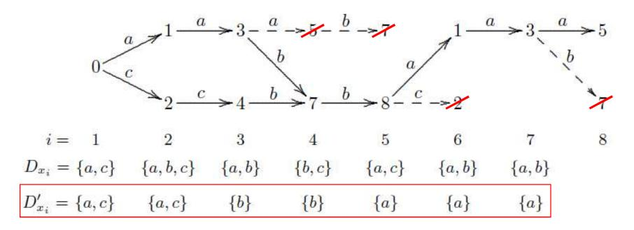
Remove states that are not backward reachable from an accepting state in the final stage.
