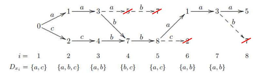
Remove states that are not backward reachable from an accepting state in the final stage.
