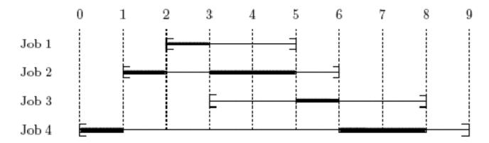
One  $O(n^2)$  algorithm is based on the Jackson pre-emptive schedule (JPS). Using a different example, the JPS is:
