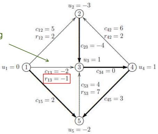
Can improve solution by adding arc with negative reduced cost to basis.
